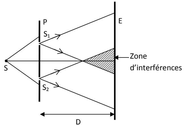
Vibration issue de  $S_1 \rightarrow Y_1(M) = S_0 \sin \omega(t - \frac{d_1}{c})$
